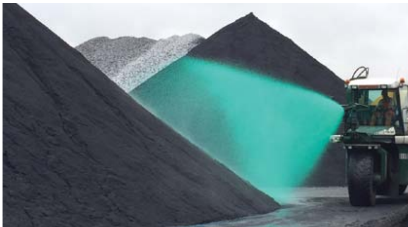
FOT. 2 Application of EcoCrust with spray tank.
